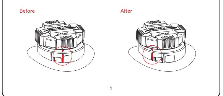
3. Ensure this step 2 is done correctly before disassembly, as shown in red part. 4. Hold firmly the knob and pull it up to disassemble it from the base.
