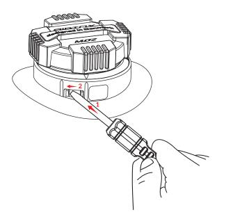
2. Then, the arrow on the knob will get aligned with the arrow at the bottom left side of the base.
