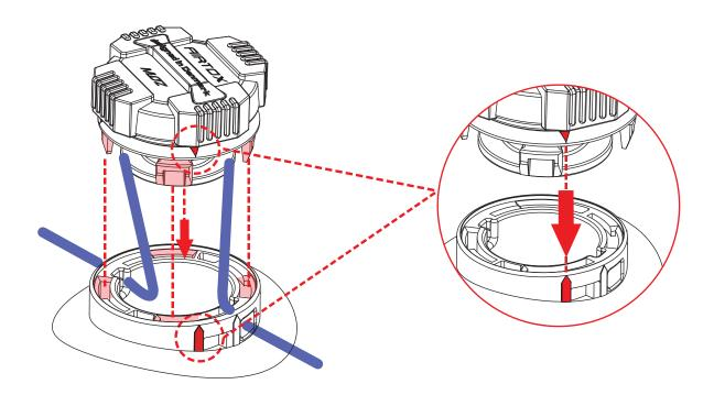
b. Turn the knob on the counterclockwise, and ensure that the arrow on the top knob and the one on the base are aligned. After you hear the "Click" sound, this means that the procedure is done.
