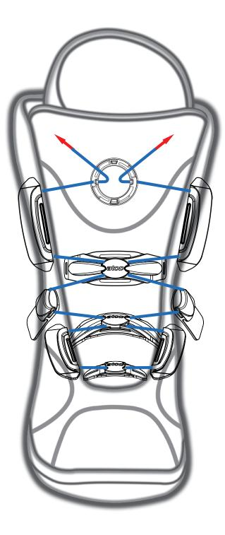
2. Turn the knob and align the arrows to any of the four hooks.
