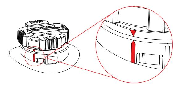
• 4. Hold firmly the knob and pull it up to disassemble it from the base.
