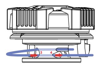
(4) Thread wire's terminal back to hole 4 to the bottom
